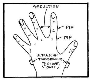
Figure 2 Flex and ultrasonic transducer placement
